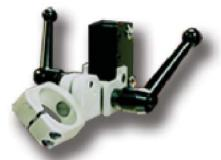
The multi position Tool Holder is standard on all TITANMATE® Tool Support Arms. The clamping mechanism is machined to fit your power tool, which gives you a full 360 degrees of tool support to prevent slippage or damage. The pivot block and clamp can be independently adjusted to any angle. Once in position these components are securely locked into position by a set of spring loaded handles. Once locked, the handles can be moved out of the way for additional clearance.
