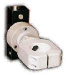
The rigid tool holder is standard on all TITANMATE® TML2-26 Support Arms. The tool holder is adjustable for the purpose of squaring the mount to the work surface. Three adjusting screws change the angle of the tool holder. Once the desired position is obtained, the mount can then be locked to prevent change in angle. The TML2-26 can also be equipped with a multi positional motor mount.
